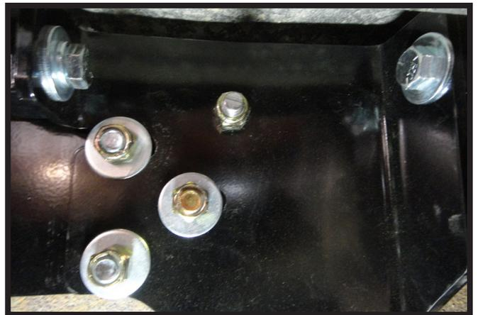
8. Install both side plates onto the cross members with the appropriate hardware. Do not fully tighten hardware.
