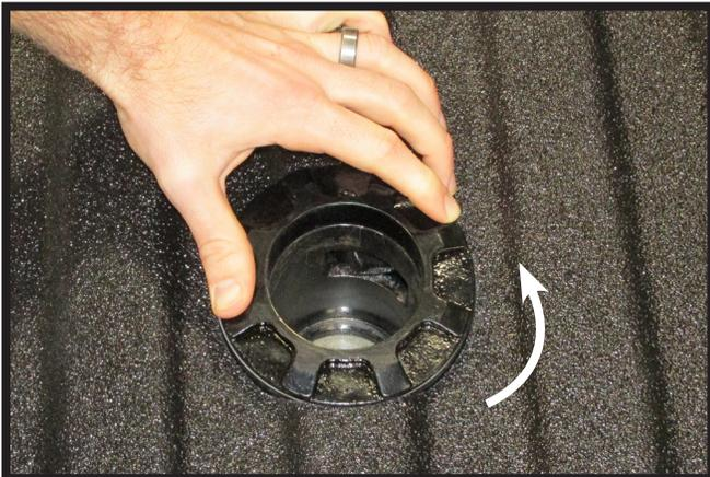
11. Check the rotation of the top collar at this time to insure the bed is not rubbing against it and it can rotate freely. If necessary drop the center section and remove any obstructions.
