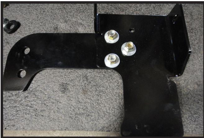
7. Install the rear plates onto the driver side and passenger side side plates with the 1/2" carriage bolts and hardware. Do not fully tighten hardware.
