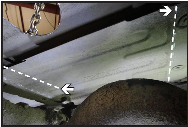
3. Remove the heat shield by cutting between two (2) bed frame rails on the underside of the bed above the axle (as shown by the dotted lines).
