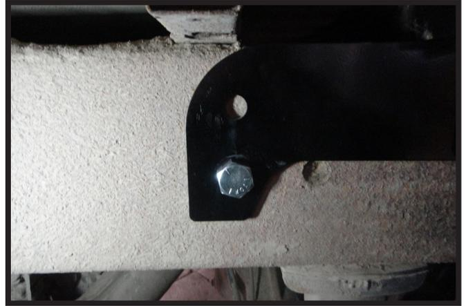
10. Adjust the rear plate if needed and install the 3/4" bolt thru the frame with the oval bushing and 3/4" hardware on the inside of the frame. Do this on both sides of the vehicle. Do not fully tighten hardware.
