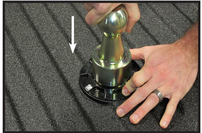
2. Align the ball with the collar and drop the ball into the hitch. Release the locking collar. Pull up on the ball to insure it is locked into the housing.
