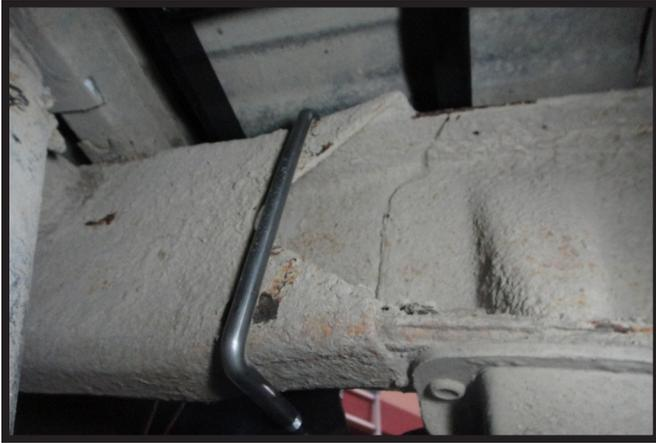
9. Install the u-bolt around the frame thru the side plate and loosely install the lock nut. Do this on both sides of the vehicle. Do not fully tighten hardware.
