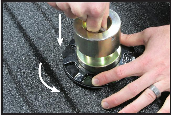
1. Rotate the locking collar to release the latch pawl. Align the ball with the collar and drop the ball into the hitch.
