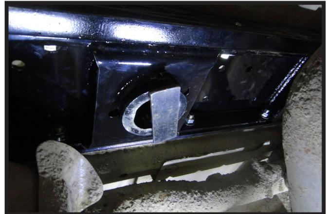
12. Tighten and torque all bolts. First torque the 3/4" bolts. Then torque the outside 1/2" bolts and work in to the 1/2" center section bolts.
