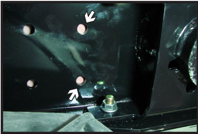
13. Using a 19/32" drill bit, drill the two (2) holes closest to the ball thru the bed. Do this on both sides of the center section.
